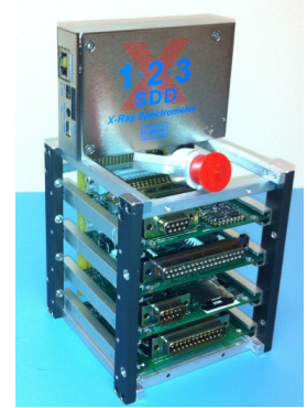
Figure 6. The X123-SDD X-ray Spectrometer is shown with the CubeSat Card Cage. These flew successfully on NASA rocket on June 23, 2012.
